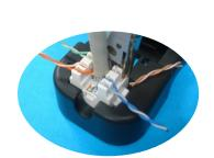
Punch the wires with 110 or Krone impact tool and cut off the surplus wires. Cap
